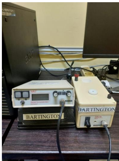
Figure 3. Bartington Magnetic Susceptibility Meter with Sensor Type B (MS2B) in Physics Laboratory, FMIPA, Universitas Negeri Padang.
